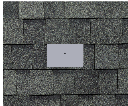
Image 5.1.2 Position flashing under shingles
