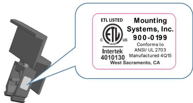
Image 1.4.1 UL 2703 system label and location
